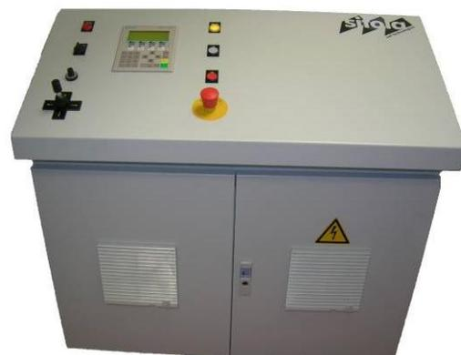
**Figure 9: New control unit of the vertical cutting machine**
