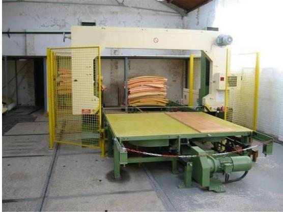
**Figure 4: Horizontal stacking machine**
