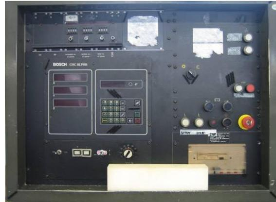
Figure 7: Old machine control of a CNC contour cutting machine
