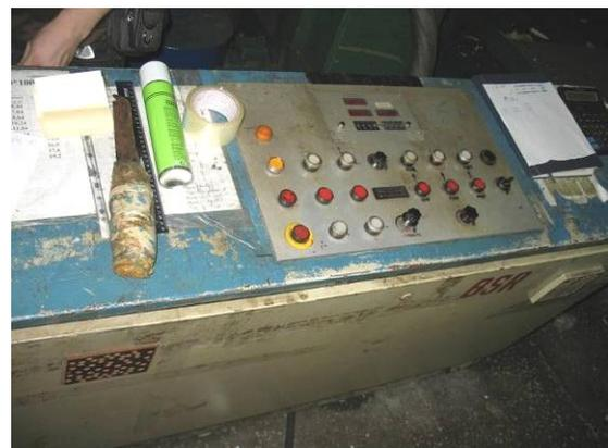
**Figure 5: Old machine control of a horizontal splitting machine**
