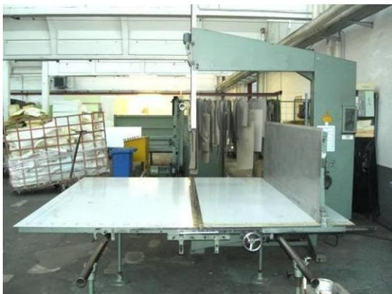
**Figure 3: Vertical cutting machine**
