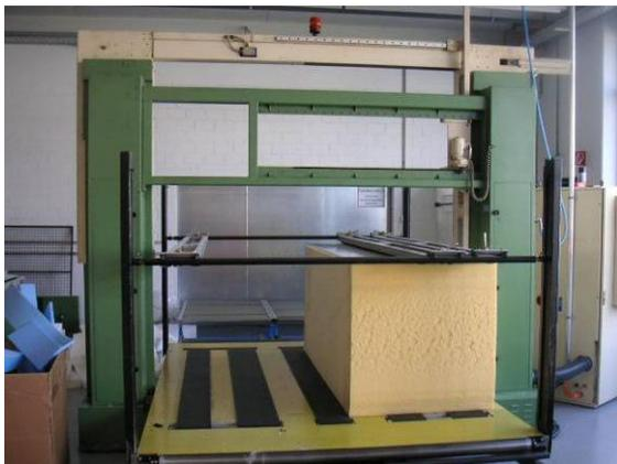
**Figure 6: CNC contour cutting machine**
