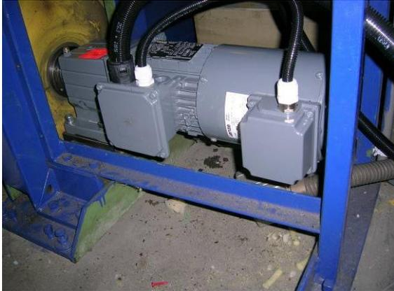
**Figure 8: Replacement motor for cutting machine**
